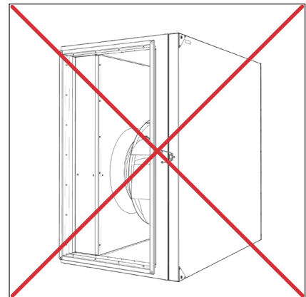
Installed with lid facing to the side.
